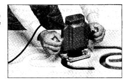
To install the templet guide, loosen the screws on the tool base, insert the templet guide and then tighten the screws.
